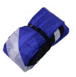
Step 5: Fold the sack as shown in the photo. This method is very gentle to the more stiffer parts of the glider.
