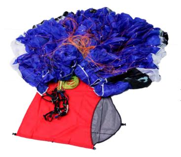
Step 1: Open the folding bag and pull the partially in. The outside will look like a cabbage. This way you're avoiding that the glider drags over the ground during folding.
