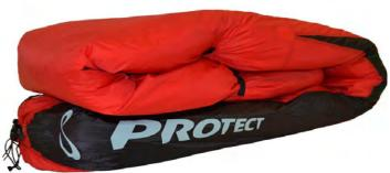
Step 5: At last fold the sack as shown in the photo. This method is very gentle to the more stiffer parts of the glider.
