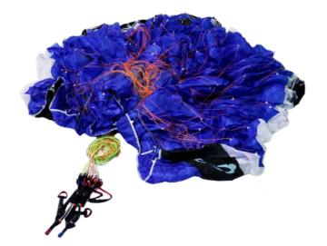
Step 1: Bundle up your glider in form of a cabbage. This way you're avoiding that the glider drags over the ground during folding.
